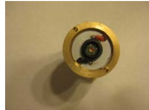
This is the proper placement of washer onto LED
