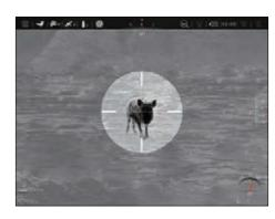
time to turn on or off the ROI feature. A circular high-contrast, high-brightness region will appear in the center of the screen.
